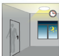
3. After elapse of hold time, the sensor dims the light at a low light level if no new motion is detected.
